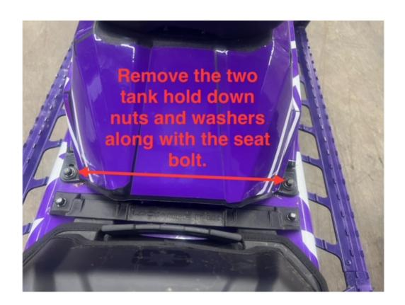
**3)**Remove the fuel cap and tank nut. Remove the switch panel (you can either unplug the switches or move the panel out of the way).
