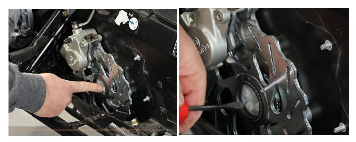
Set the plastic plug aside as you will reinstall prior to putting the brake rotor cover back on.
