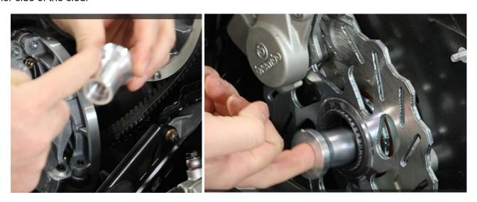
The aluminum plug will come through the shaft and line up with the edge of the inner shaft piece as shown below.
